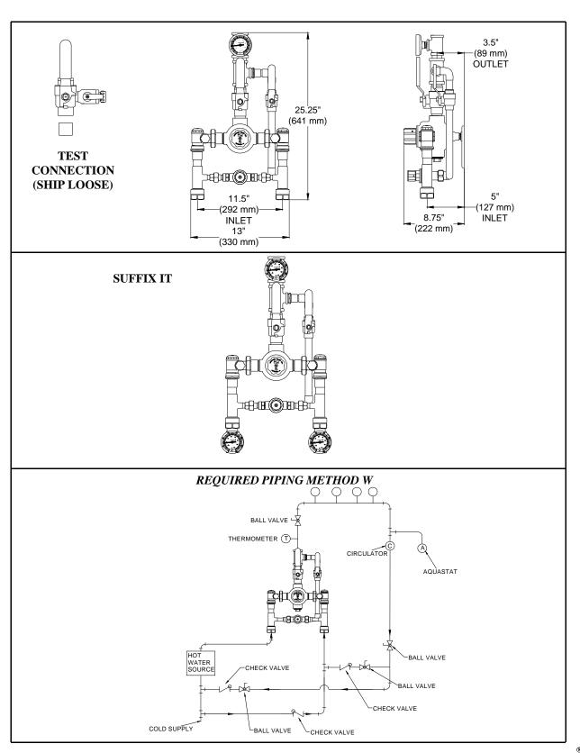
**CAUTION!** All thermostatic water mixing valves have limitations. They will NOT provide the desired accuracy outside of their flow capacity range. Consult the Flow Capacity Chart and DO NOT OVERSIZE. Minimum flow must be no less than as indicated.
